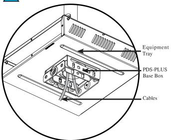
**Step 1.** Pull all cables down through the PDS-PLUS base box.
